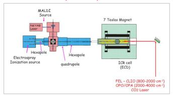
The CLIO I experiment is designed to elucidate the structure of gas phase mass-selected ions. A modified ion trap, equipped with an electrospray source, is coupled to the Free Electron laser CLIO (Centre Laser Infrarouge d'Orsay) or to an OPO/OPA to record, through an MS<sup>2</sup> experiment, the IR spectrum of the mass selected ions in the 500-3800 cm<sup>-1</sup> energy range.
